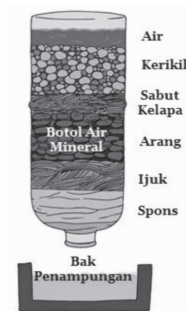
Gambar 100. Water Purification Sederhana
